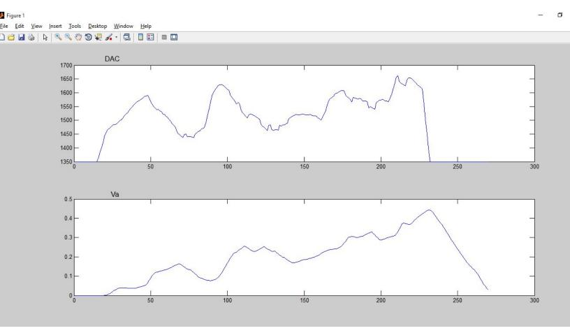
The above figure shows smoothened out data, sans any peaks. The original data on the other hand had a lot of peaks that were due to incorrect placement of the encoders on our vehicle. That was a small issue. So I used the following code in MATLAB to render the above graphs. The va value was too spiky so I had to apply it twice.
