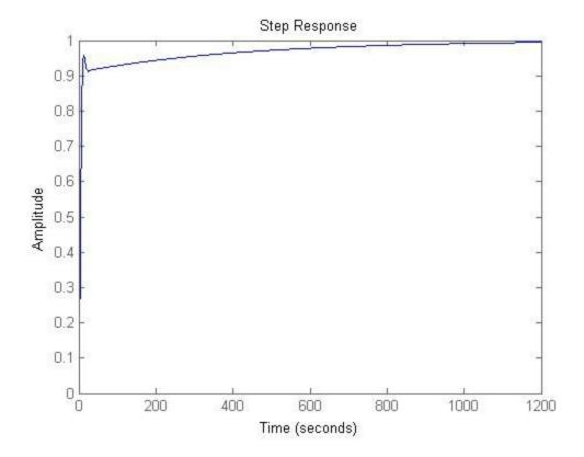
Which was really nice in the rise time and steady state error department. But as we can appreciate, the settling time is close to a 1000 seconds. The controller thus rises really fast and settles really slowly. In addition, absence of Kd leads to a lot of bumps in the real world tests and as expected the robot wasn't able to move well.
