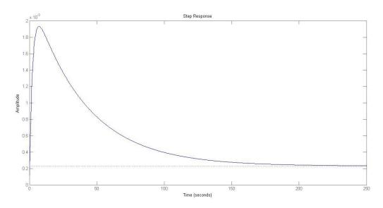
Which as we can appreciate is stable but has really high overshoot. As the input variable was the digital value feeded to DAC (in 1000s) and the output was a velocity term (in scale of e-01), we won't expect the step response to settle anywhere near 1 and that is what it did. So basically if we give a DAC value of 1, the velocity will settle down to 0.22\*10^-3 m/s, both of which are completely meaningless. So the above plot has no real significance.
